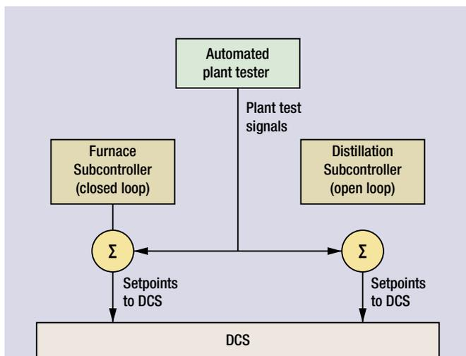
**FIG. 1** The automated tester generates plant test signals and sends them to the DCS.
