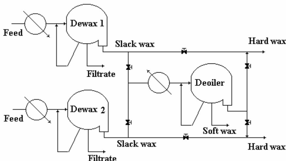
Figure 1- DEA Grasbrook Solvent Dewaxing Facilities
